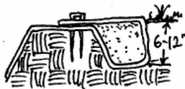
Figure 26. Keying In Diagram from The Capay Valley Conservation and Restoration Manual (Howard et al., 2002).
