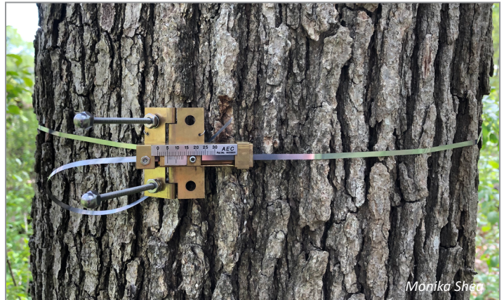
The UW Forest Ecology class will use dendrometers to measure tree growth in the Preserve as part of a long term monitoring project.
